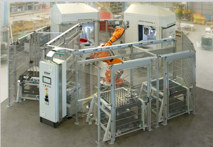
Two Rösler drag finishers R 6/1000 SF-A with robotic work piece handling
