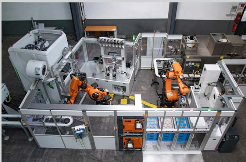
Rösler multi-surf-finisher RMSF 4/800-A integrated into a fully automated processing line. Includes work piece handling with two industrial robots, Rösler continuous flow washing machine and final quality control with marking of the finished work pieces.
