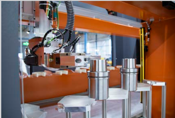
Rösler multi-surf-finisher RMSF 4/800-A with fully automated gantry loading system
