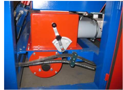
Adjustable air-flow media pre-cleaner below the barrel housing removes flashes from the parts and other impurities from the blast media
