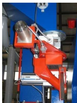
Encapsulated blast media dosing system from media hopper to blast wheel reduces the operating noise
